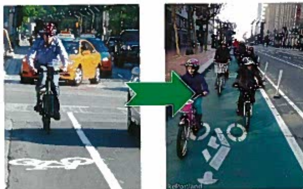
Install plastic bollards along painted bike lanes to make it clear that cars are not allowed in the cycling lane.
